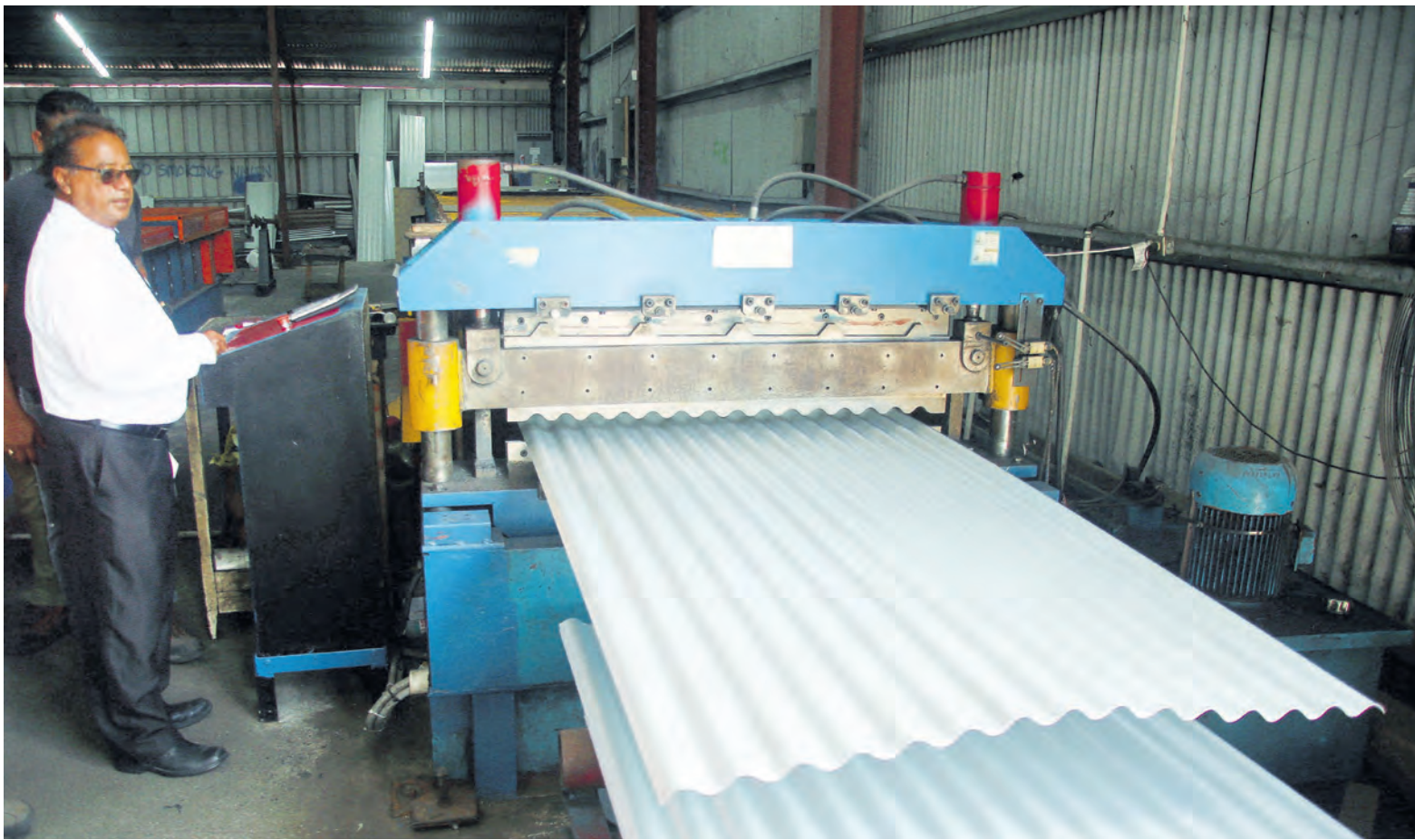
Build to Last executive director Terrence Kalloo operates a corrugated sheet roll machine. PHOTO BY LINCOLN HOLDER
